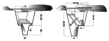
Figure 4. Trench latrine equipped with a pallet
