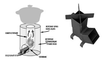
Fig. 9. Rocket stove made of two conserval cans (drainpipe) of different diameters
