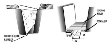
Figure 2. Drainage groove at the bottom of the trench
