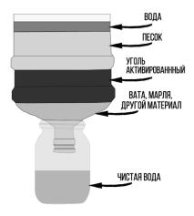
Figure 11. Filter for water purification
