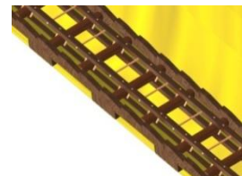
Notched wooden pieces were inserted into the mortises cut into the side benches; they allowed the rollers of the rollers-train to be held laterally and included notches of a ratchet and pawl system for the safety of the counterweight trolley.
