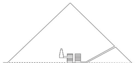
The pyramid of Huni in Meidum: The burial chamber is dug into the bedrock but its cover is a corbelled vault.
