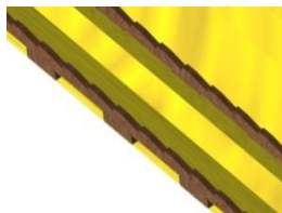
Notched wooden pieces were inserted into the mortises cut into the side benches; they allowed the rollers of the rollers-train to be held laterally and included notches of a ratchet and pawl system for the safety of the counterweight trolley.
