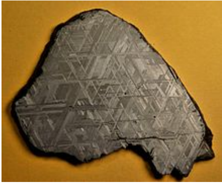
Slice (across 9.6 cm) of a Muonionalusta meteorite fragment, showing the Widmanstätten pattern .
